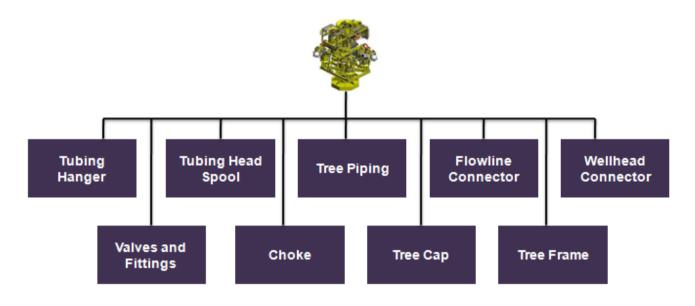
The Tubing Hanger (TH) provides means of communication between the XT and the downhole hydraulic and electric functionalities. Wet mate couplers / connectors are located on the top and bottom of the hanger and engage with the XT and downhole equipment
