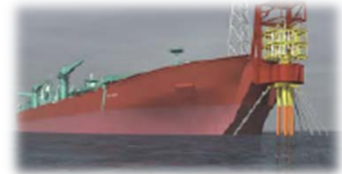
Single Point Mooring
