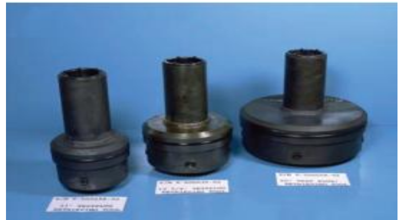
Photo of the wear bushing running tools. These tools are also used to test the BOP stack.
